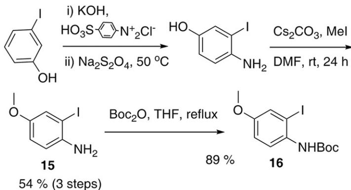
Scheme 2. Synthesis of Boc-protected 4-methoxy-2-iodoaniline.
