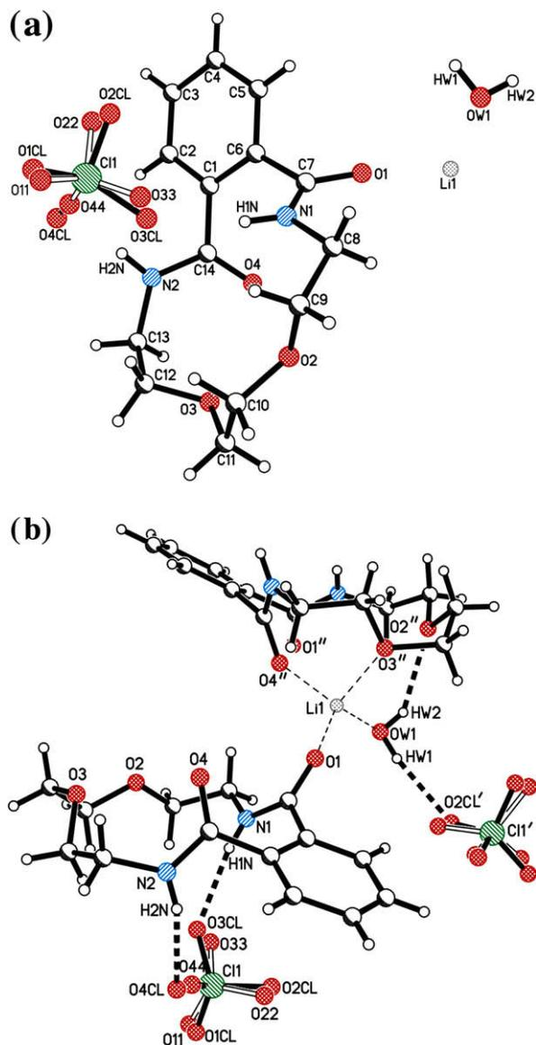
**Fig. 2.** (a) A perspective view of symmetry-independent part of the unit cell of the CPhDA–LiClO<sub>4</sub>–H<sub>2</sub>O complex; (b) a perspective view of the coordination scheme of the Li<sup>+</sup> cation. The superscripts refer to the symmetry codes in Table 2. Two sites of the orientationally disordered perchlorate anions have been shown. The hydrogen bonds have been indicated by thick dashed lines and the coordination bonds by the thin dashed lines.
