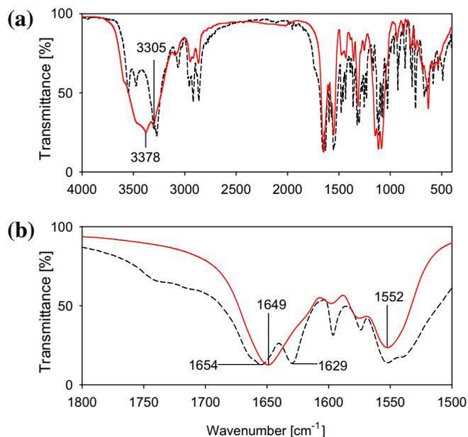
Fig. 4. The FT-IR spectra of crystal of [CPhDA-LiClO<sub>4</sub>-H<sub>2</sub>O (1:1:1)] (—) and [CPhDA-H<sub>2</sub>O (2:1)] (---) recorded in KBr pallet: (a) 4000–400 cm<sup>-1</sup>; (b) 1800–1500 cm<sup>-1</sup>.
