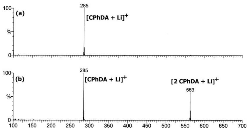
**Fig. 1.** The ESI positive ion mode mass spectra of: (a) 1:1 mixture of CPhDA with LiClO<sub>4</sub>; (b) 2:1 mixture of CPhDA with LiClO<sub>4</sub> at *cv* = 30 V.
