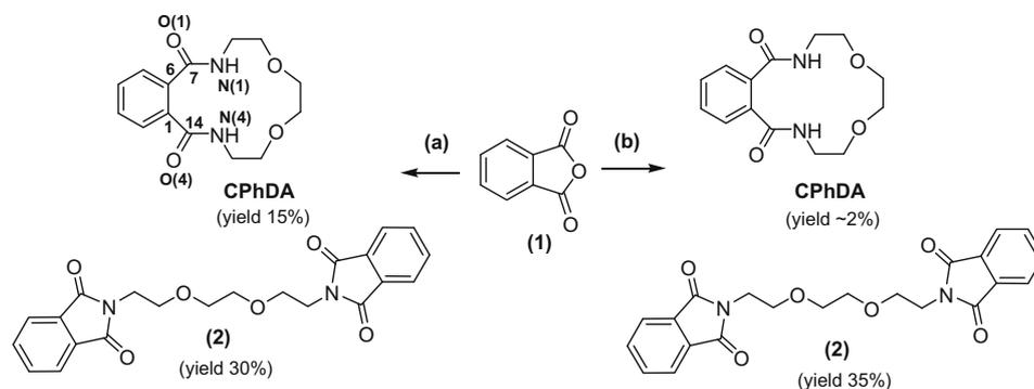
**Scheme 1.** Synthesis of cyclic diamide of *o*-phthalic acid (CPhDA). Reagent and conditions: (a) *o*-phthalic anhydride (**1**) (1.0 equiv), 1,2-bis(2-aminoethoxy)ethane (1.0 equiv), toluene, 100 °C, 24 h; (b) *o*-phthalic anhydride (**1**) (1.0 equiv), 1,2-bis(2-aminoethoxy)ethane (1.0 equiv), lithium perchlorate (2.0 equiv), acetonitrile, 80 °C, 24 h.
