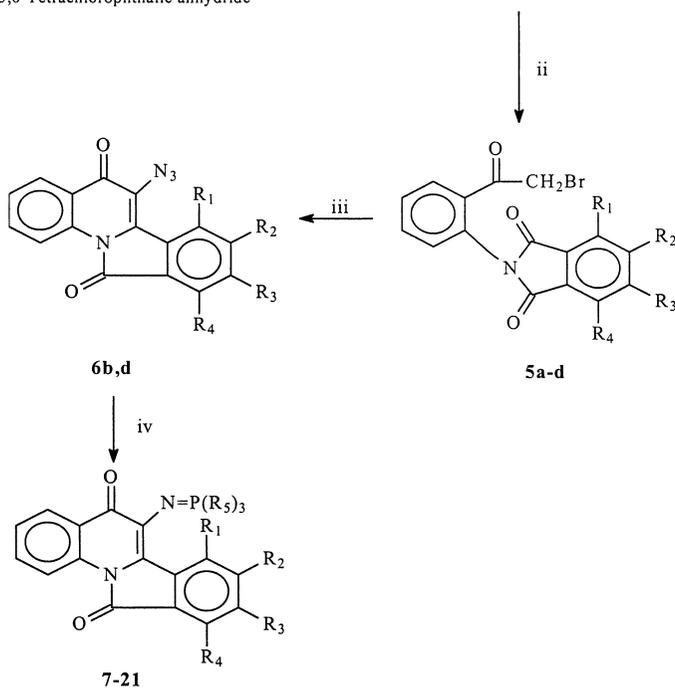
Conditions: i: xylene, Et<sub>3</sub>N, reflux; ii: CuBr<sub>2</sub>, EtOAc, CHCl<sub>3</sub>, reflux; iii: NaN<sub>3</sub>, H<sub>2</sub>O, acetone; iv: (R<sub>5</sub>)<sub>3</sub>P, THF, reflux.
