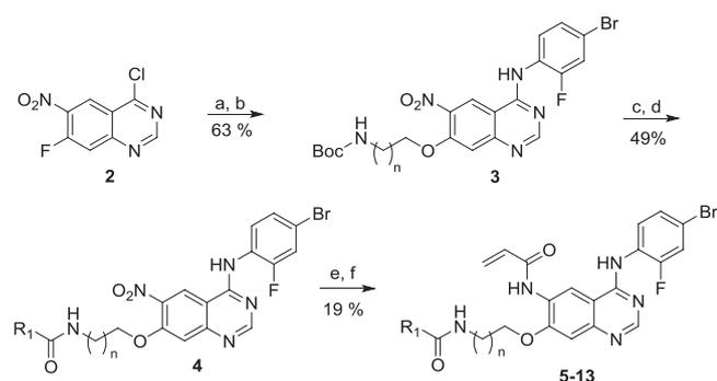
**Scheme 1.** (a) 4-bromo-2-fluoroaniline, iPrOH, reflux, 4 h; (b) *N*-Boc amino alcohol, KOTMS, DMSO, rt., 4 h; (c) TFA, CH<sub>2</sub>Cl<sub>2</sub>, rt., 0.5 h; (d) R<sub>1</sub>CO<sub>2</sub>H, EDCl, pyridine, rt., 4 h; (e) Fe, AcOH, reflux, 2 h; (f) acryloyl chloride, DMF, rt., 1 h.
