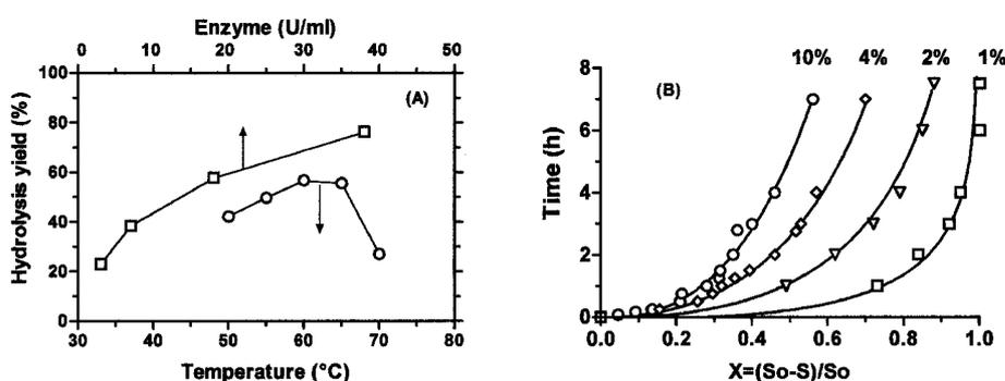
Fig 4. Hydrolysis of Supersaturated Naringin Solutions. A) Effects of temperature and enzyme level on yield after 4 hours of hydrolysis.  $\square$ : 4% naringin, 60°C;  $\circ$ : 10% naringin, 7 U/ml B) Effects of initial substrate concentration at the necessary time to reach different conversions. Symbols: experimental points; lines: theoretical curves obtained with eq. 8 and 9.
