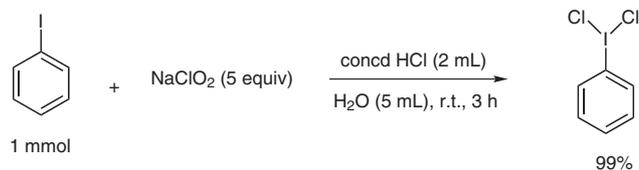
**Scheme 4** Optimal reaction conditions for the preparation of iodoarene dichloride by sodium chlorite
