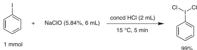
**Scheme 5** Optimal reaction conditions for the preparation of iodobenzene dichloride by sodium hypochlorite
