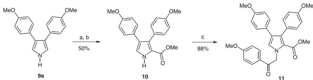
**Scheme 2** Acylation and N-alkylation of pyrroles. *Reagents and conditions:* a) ClCOCCl<sub>2</sub> (1.5 equiv), DMAP (1.6 equiv), 25 °C, 3 h; b) NaOMe (4 equiv), MeOH, 25 °C, 24 h; c) K<sub>2</sub>CO<sub>3</sub> (8 equiv), 2-bromo-4'-methoxyacetophenone (2 equiv), acetone, reflux, 3 h.
