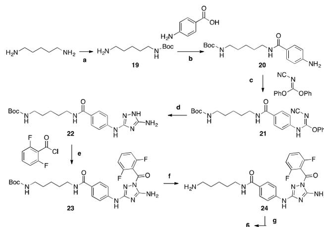
**Reagents and conditions:** (a) (Boc)<sub>2</sub>O, DCM, rt, 20 h; (b) Py-BOP, HOBT, Et<sub>3</sub>N, THF, rt, 20 h; (c) THF, 65 °C, 20 h; (d) hydrazine, THF, 70 °C, 2 h; (e) Py, rt, 18 h; (f) THF, TFA, 50 °C, 3 h; (g) Fluorescein-NCS, DIPEA, DMF, rt, 1 h.
