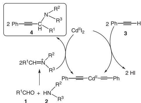
**Scheme 2** Plausible mechanism for the cadmium-catalyzed synthesis of propargylamines
