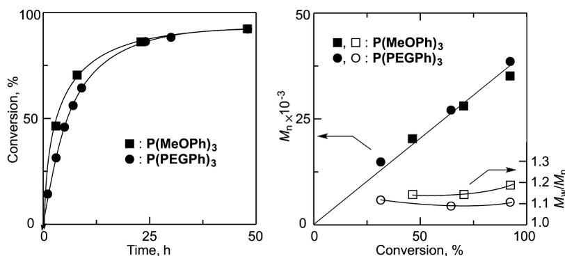
Figure 5. Conversion vs  $M_n$  and  $M_w/M_n$  plots for iron-catalyzed LRP of PEGMA with  $P(\text{PEGPh})_3$  or  $P(\text{MeOPh})_3$  as a ligand in toluene at 60 °C:  $[\text{PEGMA}]_0/[\text{H}(\text{MMA})_2\text{Br}]_0/[\text{Fe-complex}]_0 = 500/5/5$  mM. Fe-complex was prepared in prior to polymerization via aging process of  $\text{FeBr}_2$  and 2 equiv of phosphine ligand in toluene at 60 °C in 12 h and directly employed without purification.
