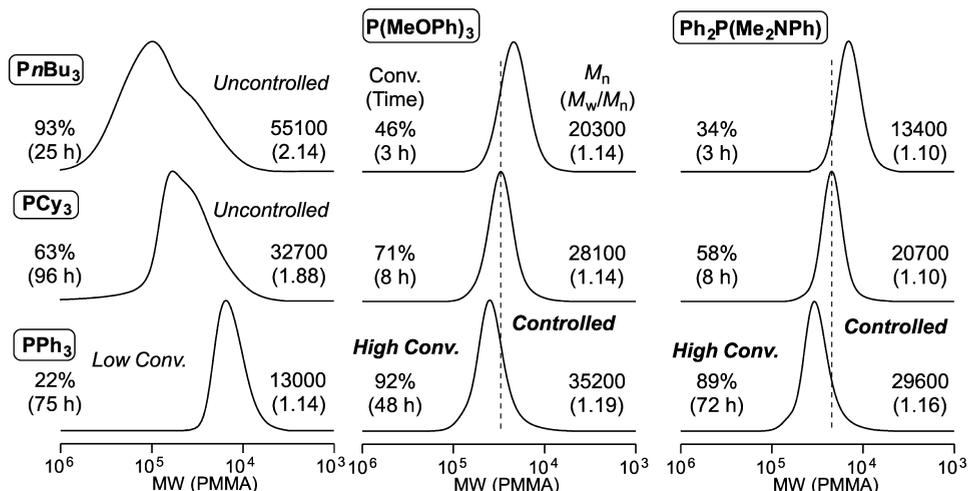
**Figure 2.** SEC curves of obtained polyPEGMA to see effects of ligand on molecular weight control in iron-catalyzed radical polymerization of PEGMA. Polymerization conditions: see caption of Figure 1.
