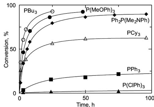
**Figure 1.** Effects of phosphine ligand on polymerization rate of iron-catalyzed polymerizations of PEGMA in toluene at 60 °C: [PEGMA]<sub>0</sub>/[H(MMA)<sub>2</sub>Br]<sub>0</sub>/[Fe-complex]<sub>0</sub> = 500/5/5 mM. The Fe complex was prepared in prior to polymerization via aging process of FeBr<sub>2</sub> and 2 equiv of phosphine ligand in toluene at 60 °C in 12 h and directly employed without purification.
