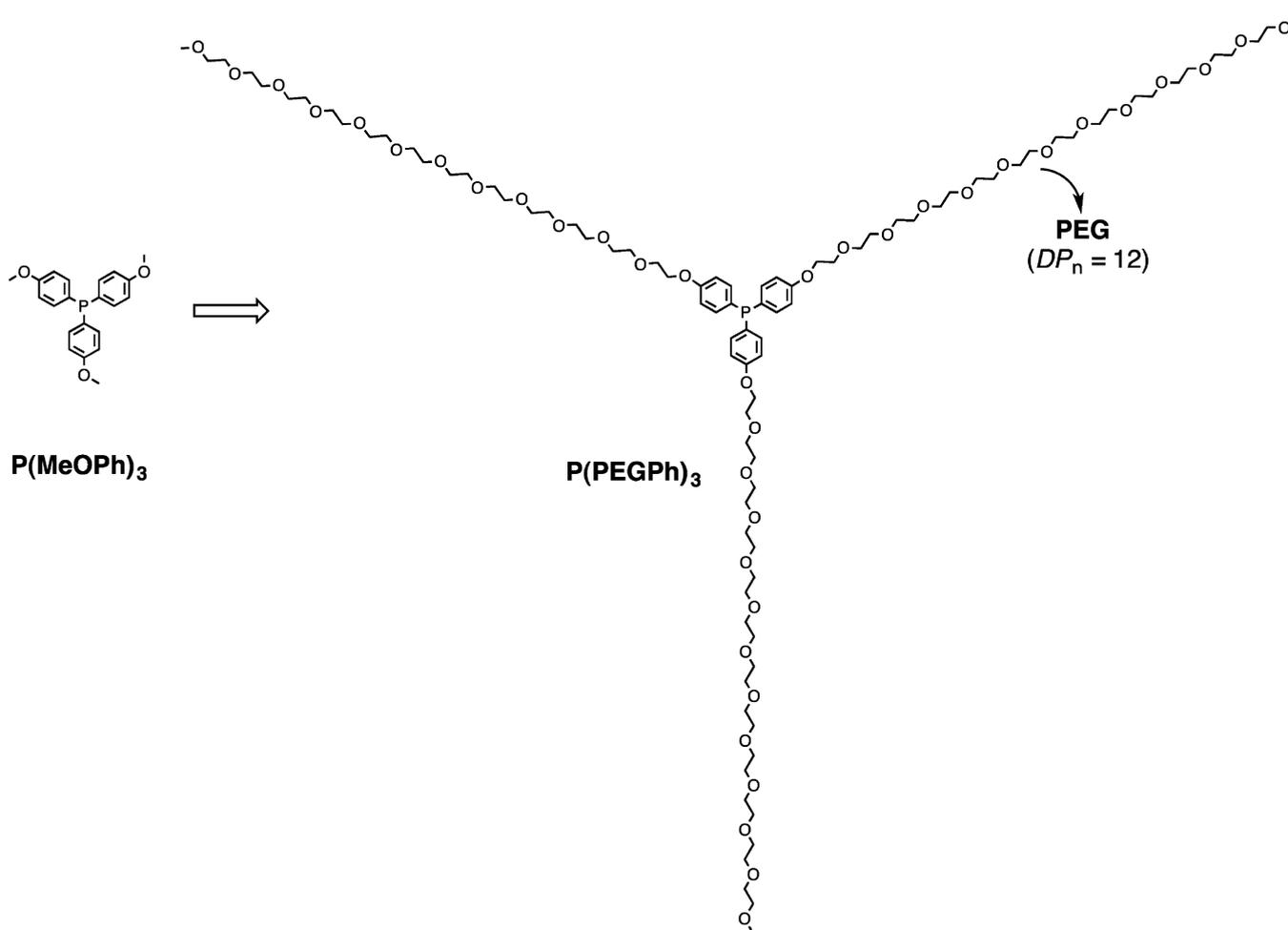
Figure 4. Decoration of *para*-substitution of triphenylphosphine with PEG chain.
