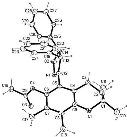
Figure 2. Thermal ellipsoid plot (40% ellipsoids) and crystallographic atom labeling of tocopherylisoxazoline **9** (4,5-diphenyl substituents in *cis* configuration) showing only one of the two conformationally different independent molecules
