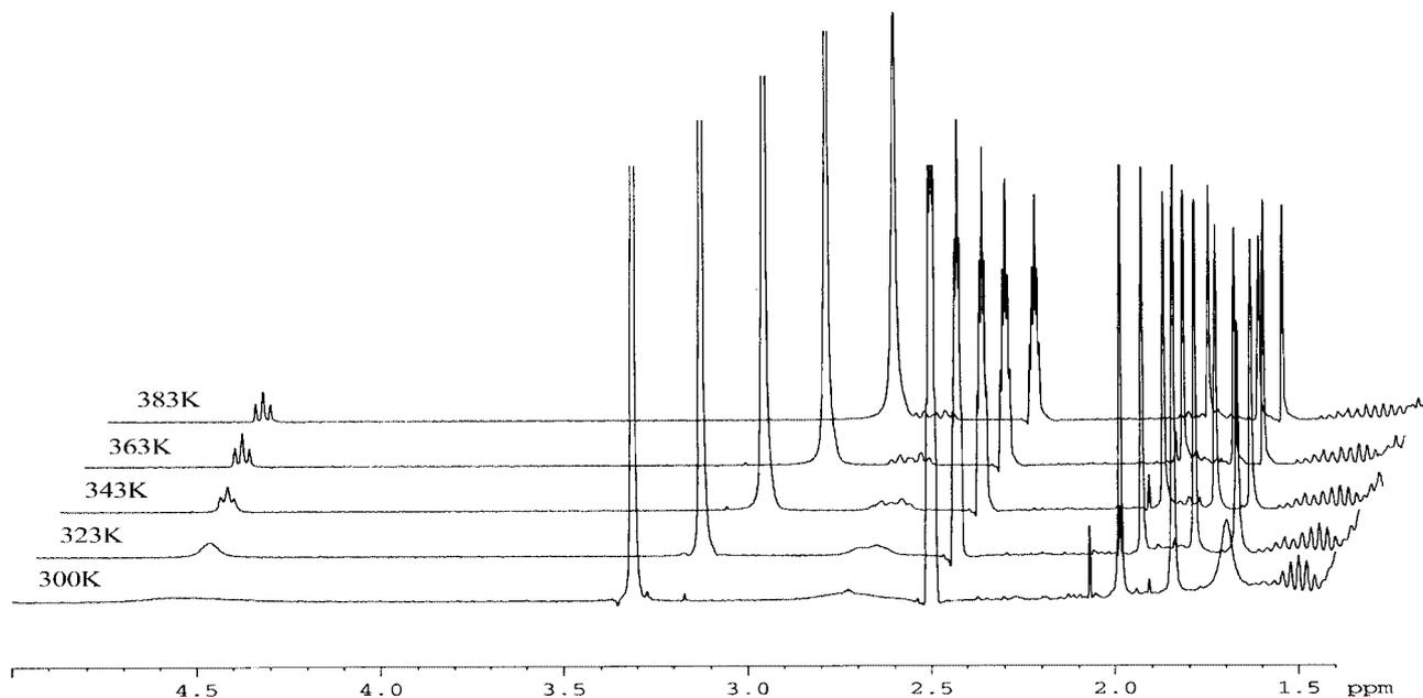
Figure 4. Stacked plots of  $^1\text{H}$  NMR spectra (region between  $\delta = 1.5$  and  $5.0$  ppm) of isoxazoline **6**, recorded at different temperatures in  $[\text{D}_6]\text{DMSO}$ ; note the temperature-dependent line shape and chemical-shift changes of the resonances of  $4''\text{-CH}$  ( $\delta \approx 4.5$  ppm),  $4\text{-CH}_2$  ( $\delta \approx 2.6\text{--}2.8$  ppm) and the acetyl group ( $\delta \approx 1.6\text{--}1.8$  ppm)
