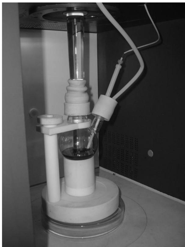
**Figure 1.** Standard set-up for simultaneous MW/US irradiation.
