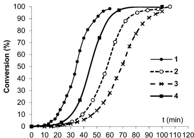
Fig. 7 RCM conversion of DEDAM with complexes 1–4 at 30 °C in dichloromethane.
