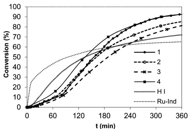
Fig. 8 RCM conversion of diethyl allyl(2-methylallyl)malonate with complexes **1–4**, **HI** and **Ru-Ind** at 30 °C in dichloromethane.
