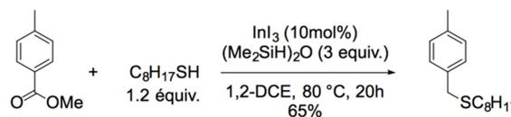
**Scheme 4.** Example of the indium(III)-catalyzed reductive sulfidation of methyl *p*-methylbenzoate with 1-octanethiol, as reported by Sakai *et al.*<sup>[18]</sup>
