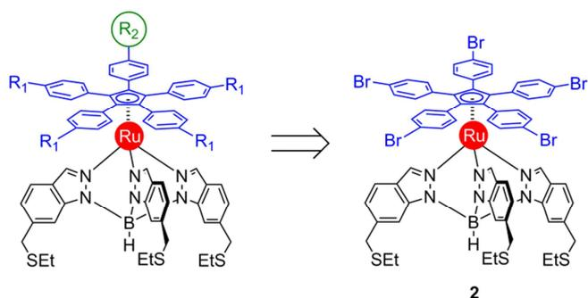
**Scheme 1.** Structure of symmetric (R<sub>1</sub> = R<sub>2</sub>) or dissymmetric (R<sub>1</sub> ≠ R<sub>2</sub>) molecular motors and gears, and related retrosynthetic analysis leading back to common key intermediate **2**.
