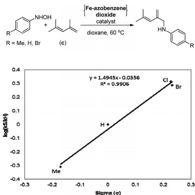
Figure 1. Hammett plot ( $k_{rel}$  vs.  $\sigma$ ) for the reaction of diene **c** with *p*-substituted phenylhydroxylamines.
