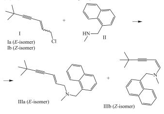
In order to ensure the complete consumption of chloroheptenyne Ia (which is the most expensive precursor) during the synthesis of terbinafine, the corresponding amine II is taken is excess. Therefore, as is naturally expected, the final reaction mass also contains this excess amine II which, after acidification with hydrochloric acid, mostly passes to the aqueous phase so that the rough target product (terbinafine) contains only trace amounts of amine II.
