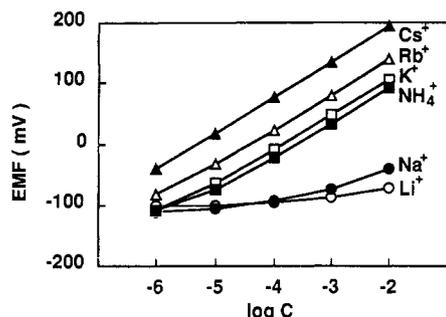
**Figure 4.** Potential vs concentration curves for alkali metal and ammonium cations, obtained at pH 7.0 by electrode 1 based on the calix[6]arene hexaester 1a. Measured in 0.1 M Tris-HCl buffer (pH 7.0) at room temperature (ca. 20 °C).
