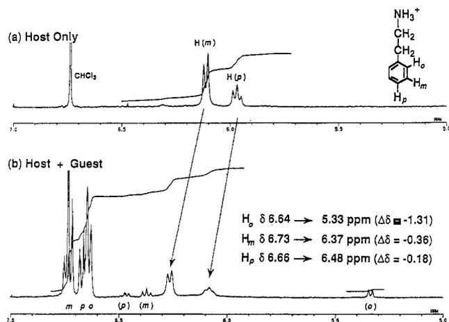
**Figure 9.** Changes in  $^1\text{H-NMR}$  spectra by the host-guest complexation between the calix[6]arene hexaester (**1a**) and 2-phenylethylamine hydrochloride (**5-HCl**) in  $\text{CDCl}_3\text{-CD}_3\text{OD}$  (90:10) at an ambient temperature of  $24 \pm 1^\circ\text{C}$ : (a)  $[\mathbf{1a}] = 1.5 \times 10^{-3}$  M. (b)  $[\mathbf{1a}] = 1.5 \times 10^{-3}$  M,  $[\mathbf{5-HCl}] = 1.5 \times 10^{-2}$  M.
