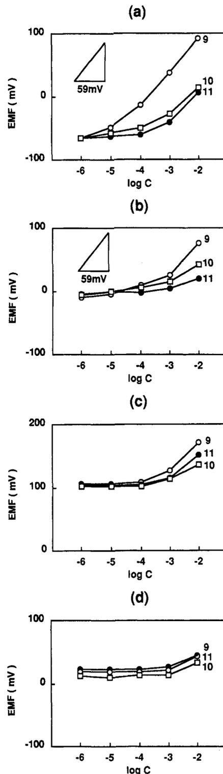
**Figure 6.** Potential vs concentration curves for catecholamines at pH 7.0: (a) Electrode **1** based on the calix[6]arene hexaester **1a**. (b) Electrode **2** based on dibenzo-18-crown-6 (**2**). (c) Electrode **3** based on potassium tetrakis(*p*-chlorophenyl)borate (**3**). (d) Electrode **4** with a membrane containing only DOS and PVC. Measured at room temperature (ca. 20 °C) in 0.1 M Tris-HCl buffer containing 0.01 M L-ascorbic acid (pH 7.0).
