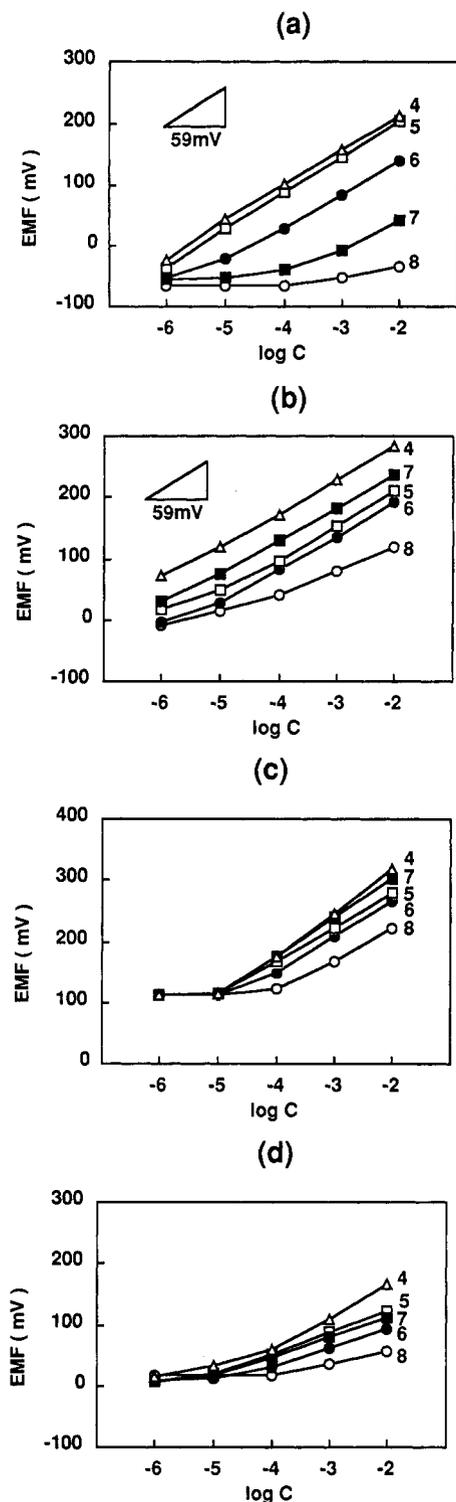
**Figure 5.** Potential vs concentration curves for simple amines at pH 7.0: (a) Electrode 1 based on the calix[6]arene hexaester 1a. (b) Electrode 2 based on dibenzo-18-crown-6 (2). (c) Electrode 3 based on potassium tetrakis(*p*-chlorophenyl)borate (3). (d) Electrode 4 with a membrane containing only DOS and PVC. Measured in 0.1 M Tris-HCl buffer (pH 7.0) at room temperature (ca. 20 °C).
