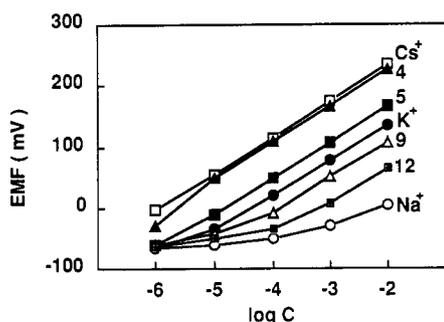
**Figure 8.** Potential vs concentration curves for representative guests of series 1–4, obtained at pH 5.0 by electrode 1 based on the calix[6]arene hexaester 1a. Measured in 0.1 M CH<sub>3</sub>CO<sub>2</sub>Li–CH<sub>3</sub>CO<sub>2</sub>H buffer (pH 5.0) at room temperature (ca. 20 °C).
