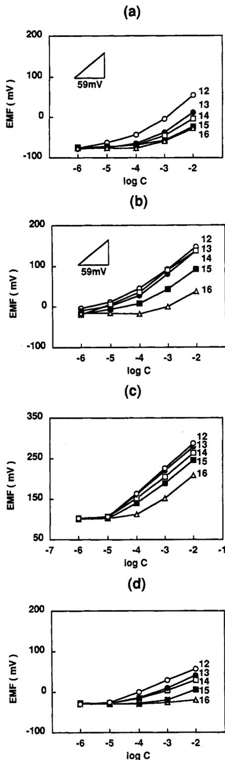
**Figure 7.** Potential vs concentration curves for  $\alpha$ -amino acid methyl esters at pH 5.0: (a) Electrode 1 based on the calix[6]arene hexaester 1a. (b) Electrode 2 based on dibenzo-18-crown-6 (2). (c) Electrode 3 based on potassium tetrakis(*p*-chlorophenyl)borate (3). (d) Electrode 4 with a membrane containing only DOS and PVC. Measured in 0.1 M  $CH_2CO_2Li-CH_3CO_2H$  buffer (pH 5.0) at room temperature (ca. 20 °C).
