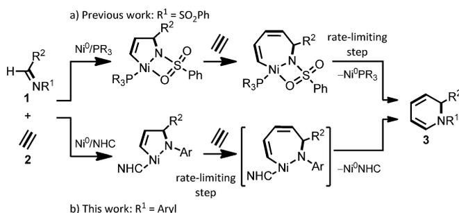
**Scheme 1.** Formation of 1,2-dihydropyridines by [2+2+2] cycloaddition of imines with alkynes in the presence of nickel(0).
