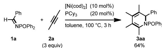
**Scheme 3.** Nickel(0)-catalyzed [2+2+2] cycloaddition of **1a** with **2a**. Yield of **3aa** was determined by <sup>1</sup>H NMR spectroscopy.
