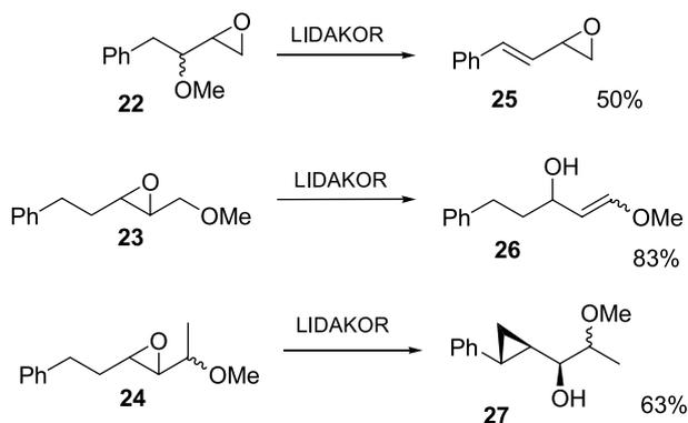
**Scheme 8.** Reaction conditions: 2 equiv LIDAKOR, THF,  $-50^{\circ}\text{C}$ , 16 h.
