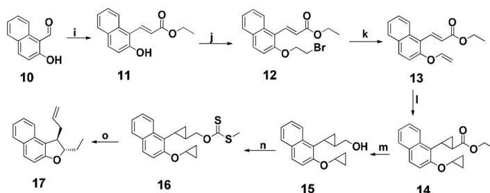
**Scheme 3.** Reagents and conditions: (i) ethyl 2-(triphenylphosphoranylidene) acetate, toluene, 0 °C → RT, 3 h; (j) 1,2-dibromoethane, K<sub>2</sub>CO<sub>3</sub>, acetone, reflux, 6 h; (k) DBU, THF, reflux, 6 h; (l) CH<sub>2</sub>N<sub>2</sub>, Pd(OAc)<sub>2</sub>, Et<sub>2</sub>O, 0 °C → RT, 1 h; (m) LAH, THF, 0 °C → RT, 5 h; (n) NaH, CS<sub>2</sub>, MeI, THF, 0 °C → RT, 18 h; (o) TBTH, AIBN, toluene, reflux, 3.5 h.
