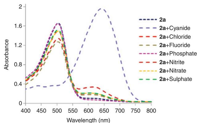
**Figure 3** Absorption spectra of  $5 \times 10^{-6}$  M solutions of 2,2-difluoro-4,6-bis[ $\beta$ -(4-hydroxy-3-methoxystyryl)]-1,3,2-dioxaborine (**2a**) in presence of 100 molar excess of various ions in MeCN/H<sub>2</sub>O (4:1).
