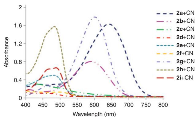
**Figure 2** Absorption spectra of  $5 \times 10^{-6}$  M solutions of curcuminoid 2,2-difluoro-1,3,2-dioxaborines **2a–i** in presence of 100 molar excess of cyanide ion in MeCN/H<sub>2</sub>O (4:1).
