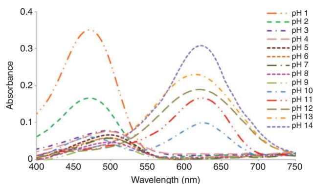
**Figure 4** Absorption spectra of 2,2-difluoro-4,6-bis[ $\beta$ -(4-hydroxy-3-methoxystyryl)]-1,3,2-dioxaborine (**2a**) in MeCN/H<sub>2</sub>O (4:1) solutions of pH range 1–14.
