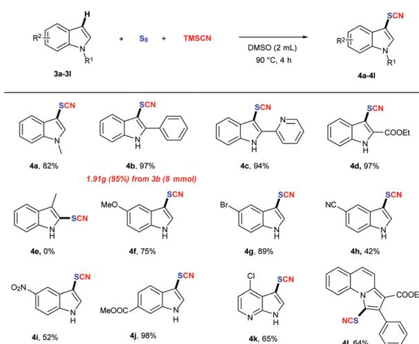
Scheme 3 C–H thiocyanation of indoles. Reaction conditions: **3** (0.2 mmol), S<sub>8</sub> (2 equiv., 0.4 mmol), TMSCN (2 equiv., 0.4 mmol), DMSO (2 mL), 90 °C, 4 h.
