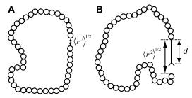
Figure 3. Random-coil polymer with the number (n) of repeat units (represented as open circles) equal to 45. (A) The polymer forms a closed loop: the distance  $(\langle r^2 \rangle^{1/2})$  between the ends of the polymer is near zero. (B) The polymer bears a physical pole of length d attached at one end. The distance  $(\langle r^2 \rangle^{1/2})$  between the ends of the polymer is close to this defined distance (d).
