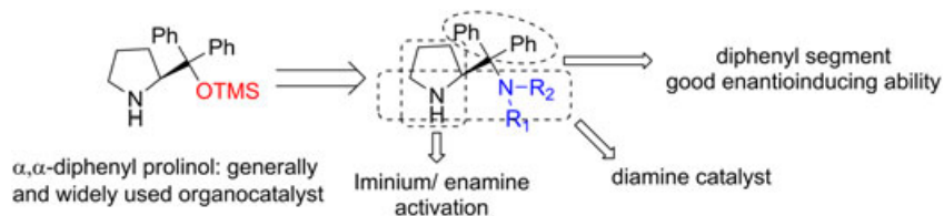
FIGURE 1 From \alpha, \alpha -diphenylprolinol silyl ether to diamine catalysts, general activation mode of diamine catalyst
