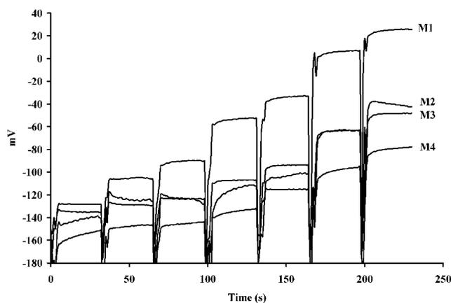
Figure 3. Potentiometric responses of planar ISEs to  $\text{NH}_4^+$  ( $10^{-4}$ – $10^{-1}$  M) for membranes 1–4 based on **IV**.
