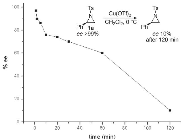
**FIGURE 2.** Racemization of (*R*)-**1a** in the presence of  $\text{Cu}(\text{OTf})_2$  in  $\text{CH}_2\text{Cl}_2$  without any nucleophile.
