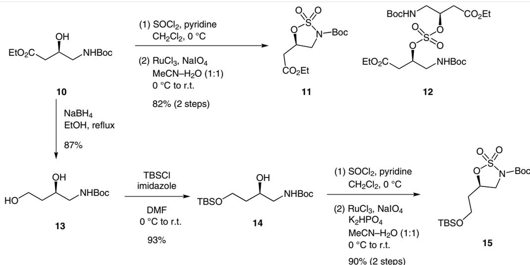
**Scheme 3** Synthesis of the key 1,2-cyclic sulfamidates **11** and **15**
