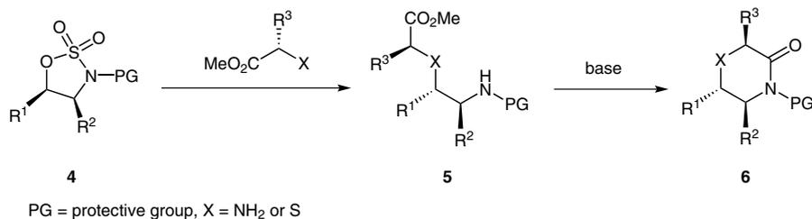
**Scheme 1** Heterocycle-formation reactions using 1,2-cyclic sulfamidates
