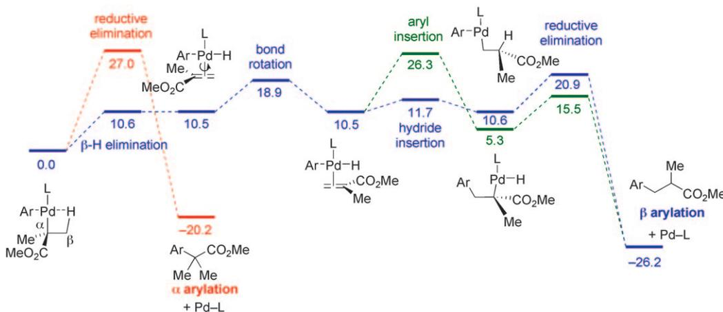
**Figure 1.** Gibbs free energy ( $\text{kcal mol}^{-1}$ ) diagram for the  $\alpha$ - and  $\beta$ -arylation pathways ( $L = \text{PCy}_3$ ,  $\text{Ar} = 2$ -fluorophenyl).
