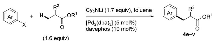
a) Scope with respect to the (hetero)aryl halide ( $R^1 = \text{Me}$  or  $t\text{Bu}$ ,  $R^2 = \text{Me}$ )
