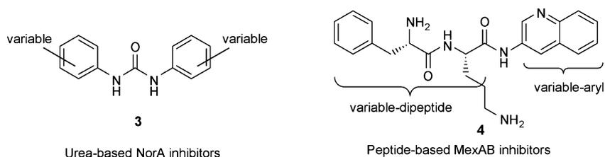
Fig. 2. Representative structures for the two classes of EPIs employed in this study. Structural variations in the aryl rings of bisaryl urea NorA inhibitors and the dipeptide and aryl components of MexAB inhibitors are accommodated, where numerous derivatives retain inhibitory activity against the respective efflux pump systems.
