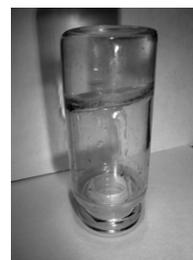
**Figure 3** Gel of (R)-(+)-**3a** in cyclohexane (a penicillin flask is turned upside down).
