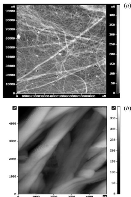
**Figure 2** AFM micrographs of the xerogels of (a) **1a** from methylcyclopentane (90x90  $\mu\text{m}$ ) and (b) **3a** from cyclohexane (5x5  $\mu\text{m}$ ). Scale to the right depicts the depth of the scan (nm) by brightness of the picture.
