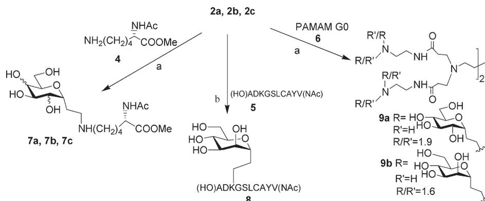
**Scheme 4:** Synthesis of derivatives **7**, **8**, and **9** by reductive amination. Reagents and conditions: a) MeOH, NaCNBH<sub>3</sub>, AcOH; b) MeOH/H<sub>2</sub>O, NaCNBH<sub>3</sub>, AcOH.
