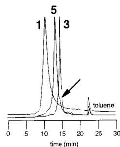
**Figure 2.** Traces were obtained on an HPLC apparatus equipped with a Jordi gel column (divinylbenzene, 500 Å pore size) using THF as a solvent (1.5 mL/min.) The retention times are 11.1 min (**1**), 13.9 min (**5**), 15.2 min (**3**).
