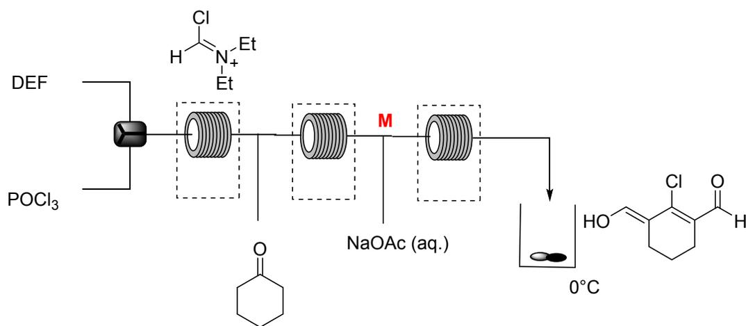
**Figure 1.** Full reaction set-up for continuous flow synthesis of compound **1**. Mixer position M is indicated in red.
