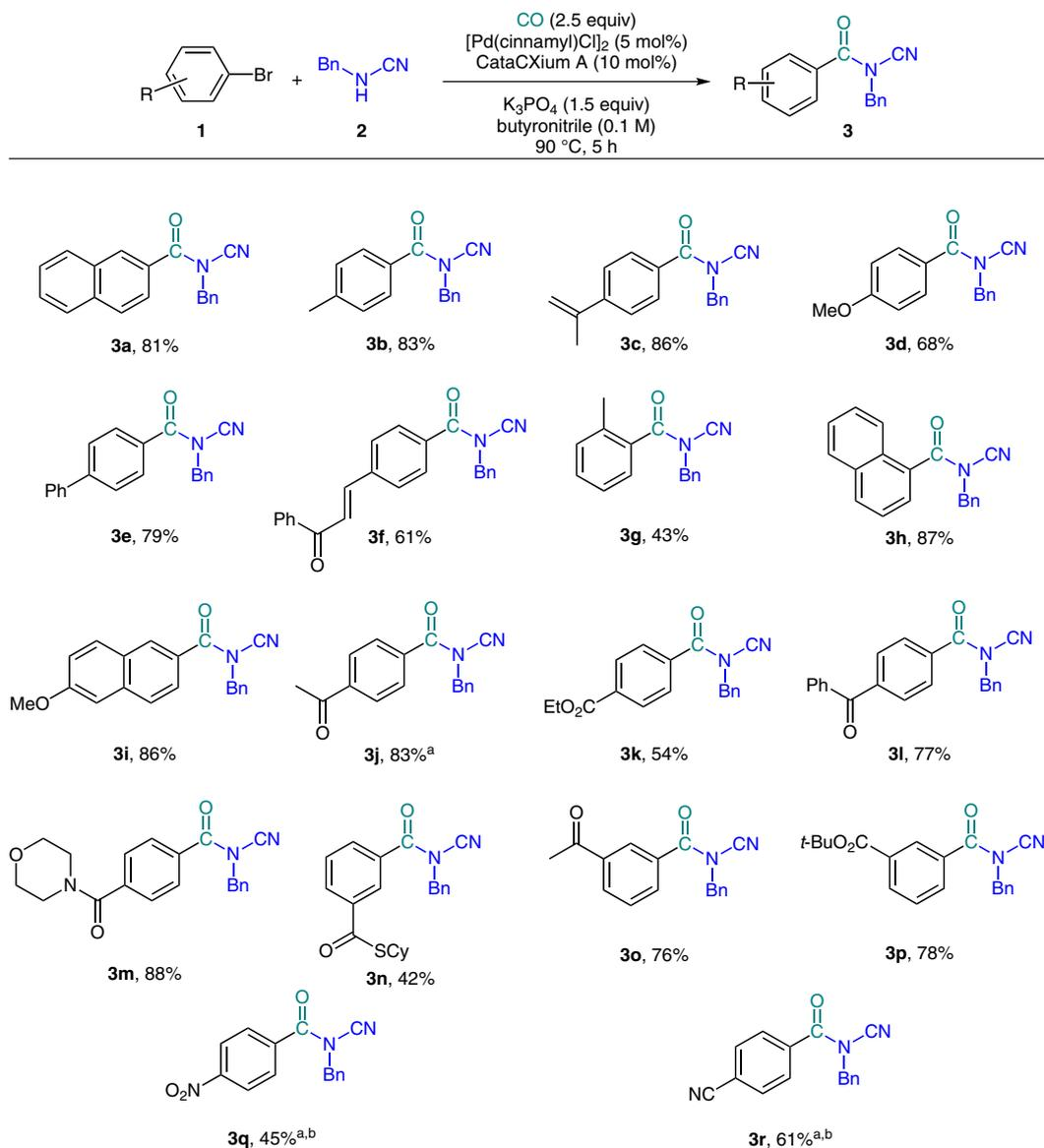
**Scheme 2** Scope of the Pd(0)-catalyzed carbonylative coupling of *N*-benzyl cyanamide with aryl bromides. (a) 80 °C. (b) [Pd(cinnamyl)Cl]<sub>2</sub> (7.5 mol%), CataCXium A (15 mol%)
