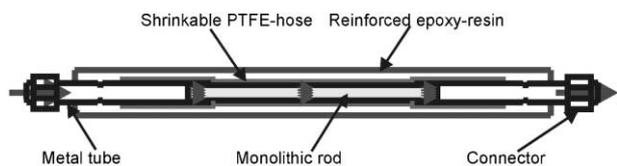
**Figure 2.** Cross sectional view through the PASSflow reactor (PTFE = polytetrafluoroethylene).
