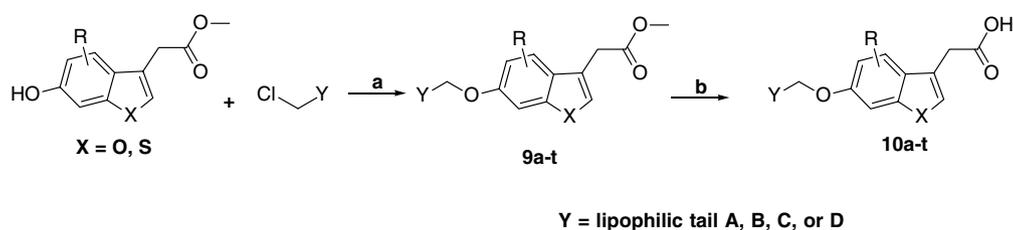
Scheme 3. Reagents and conditions: (a) Y-CH<sub>2</sub>Cl, Cs<sub>2</sub>CO<sub>3</sub>, CH<sub>3</sub>CN, 40–87%; (b) LiOH/water/THF, 55–96%.
