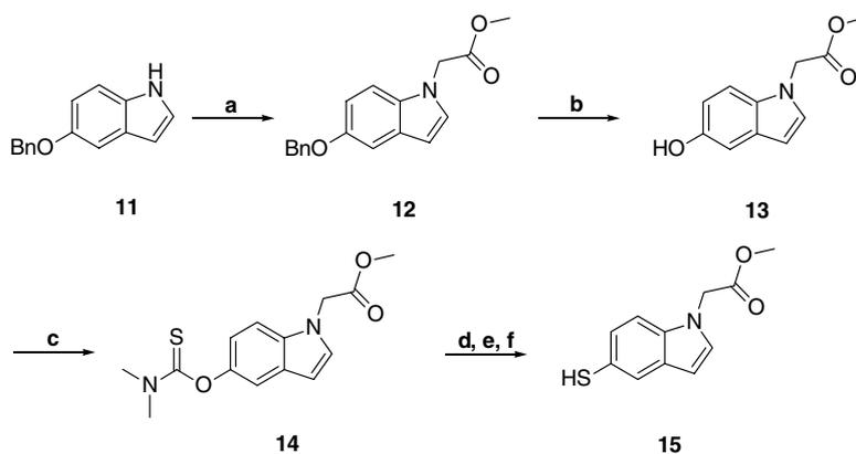
**Scheme 4.** Reagents and conditions: (a) methyl bromoacetate, NaH, CH<sub>3</sub>CN/DMF; (b) H<sub>2</sub>, 10% Pd/C; (c) *N,N*-dimethylthiocarbamoyl chloride, NaH, 39%; (d) diphenyl ether, 259 °C, 17 h, 82%; (e) KOH, ethanol, reflux; (f) MeOH, *p*-TsOH, reflux, steps (e–f) 40%.
