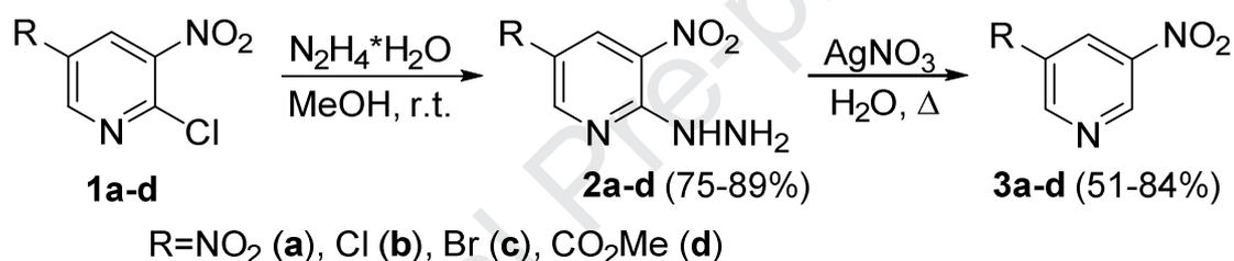
Scheme 1. Synthesis of 3-R-5-nitropyridines **3a-d**
