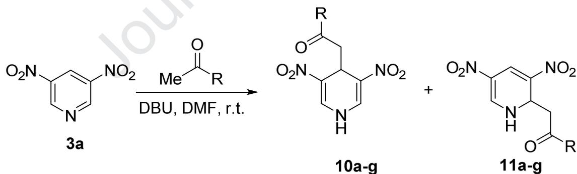
Scheme 6. Reaction of 3,5-dinitropyridine **3a** with methyl ketones
