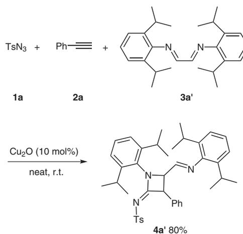
**Scheme 1** Copper(I) oxide catalyzed synthesis of azetid-2-ylidene **4a'** under neat conditions
