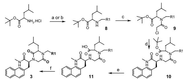
**Scheme 2.** Regents and conditions: (a) R1-CHO, Na(OAc)<sub>3</sub>BH (1.5 equiv), HOAc (0.5 equiv), THF, rt, 1 h; (b) R1-CH<sub>2</sub>Br, DIEA, DMF, rt, 16 h; (c) chloroacetic acid, DIPCl (2 equiv), DMF; (d) **4**, DIEA, DMF, 40 °C, 16 h; (e) TFA, CH<sub>2</sub>Cl<sub>2</sub>, rt, 3 h; (f) HATU (1.2 equiv), DIPEA (1.2 equiv) DMF, 0 °C–rt, 4 h.
