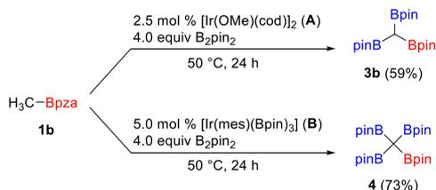
to the formation of tetraborylmethane **4** through  $\alpha,\alpha,\alpha$ -triborylation in 73% yield. To our knowledge, this is the first catalytic synthesis of tetraborylmethane.<sup>18</sup>
