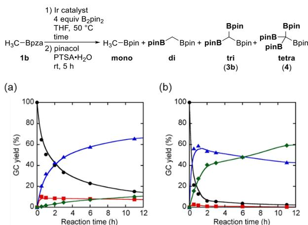
**Figure 1.** Time course for polyborylation of PZA-modified methylboronic acid with (a) 2.5 mol % of [Ir(OMe)(cod)]<sub>2</sub> and (b) 2.5 mol % of [Ir(mes)(Bpin)<sub>3</sub>]. GC yields of mono- (●), di- (■), tri- (▲), and tetraborylmethane (◆) were plotted against the reaction time.
