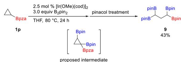
isolated 1,1,3,3-tetrakisborylpropane **9** in 43% yield through cleavage of the C–C bond in the cyclopropane ring.<sup>19</sup> Analysis of the crude mixture obtained by the reaction using 1.2 equiv of B<sub>2</sub>pin<sub>2</sub> at 50 °C for 12 h suggested the formation of 1,1,2-trisubstituted cyclopropane before the C–C bond cleavage (see the SI).
