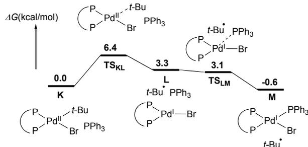
**Figure 4.** Transformation energy profile between alkyl-Pd(II) (K) and hybrid alkyl Pd(I)-radical species (M).
