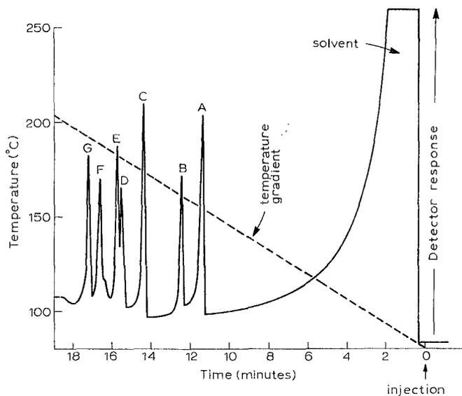
Fig. 3. Gas-liquid chromatography, on a column of 1:1 2% of OV-17-1% of OV-210 on Supelcoport, of the per-*O*-(trifluoroacetyl) derivatives of: (A) 2-acetamido-2-deoxyglycerol (1), (B) *myo*-inositol (internal standard), (C) 2-acetamido-2-deoxy-*L*-threitol (2), (D) 2-acetamido-2-deoxy-*D*-xylylitol (5), (E) 2-acetamido-2-deoxy-*L*-arabinitol (3), (F) 2-acetamido-2-deoxy-*D*-glucitol (6), and (G) 2-acetamido-2-deoxy-*D*-galactitol (4).
