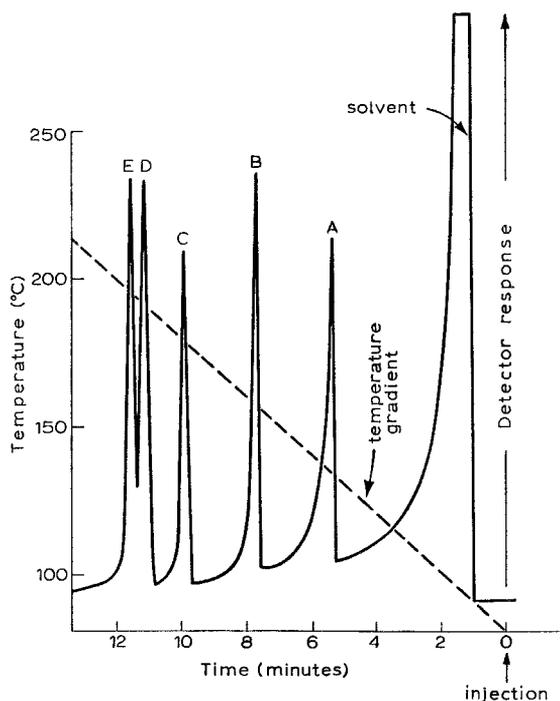
Fig. 1. Gas-liquid chromatography, on a column of 1% of OV-17 on Chromosorb GHP, of the per-*O*-(trimethylsilyl) derivatives of: (A) 2-acetamido-2-deoxyglycerol (**1**), (B) 2-acetamido-2-deoxy-L-threitol (**2**), (C) 2-acetamido-2-deoxy-D-xylitol (**5**) or -L-arabinitol (**3**), (D) *myo*-inositol (internal standard), and (E) 2-acetamido-2-deoxy-D-glucitol (**6**).
