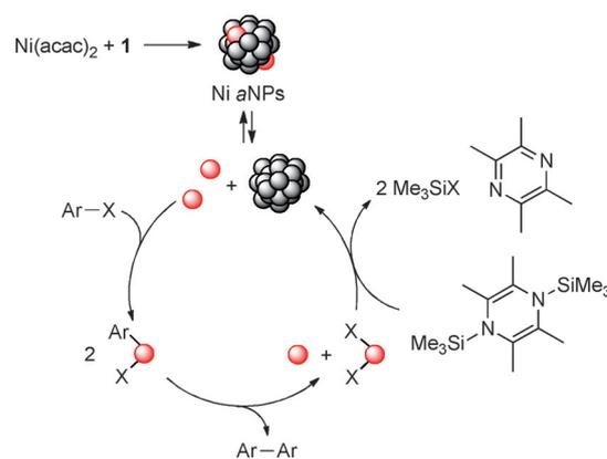
**Figure 2.** Possible reaction mechanism for reductive biaryl formation catalyzed by Ni *a*NPs.
