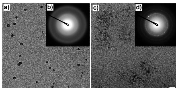
**Figure 1.** a) High-magnification TEM image and b) corresponding transmission electron diffraction (TED) pattern of Ni aNPs generated from Ni(acac)<sub>2</sub>/**1** (entry 5 in Table 2). c) High-magnification TEM image and d) corresponding TED pattern of Ni cNPs generated from NiCl<sub>2</sub>/Li/4,4'-di-*tert*-butylbiphenyl (entry 6 in Table 2). Scale bars in TEM images (bottom right) = 10 nm.
