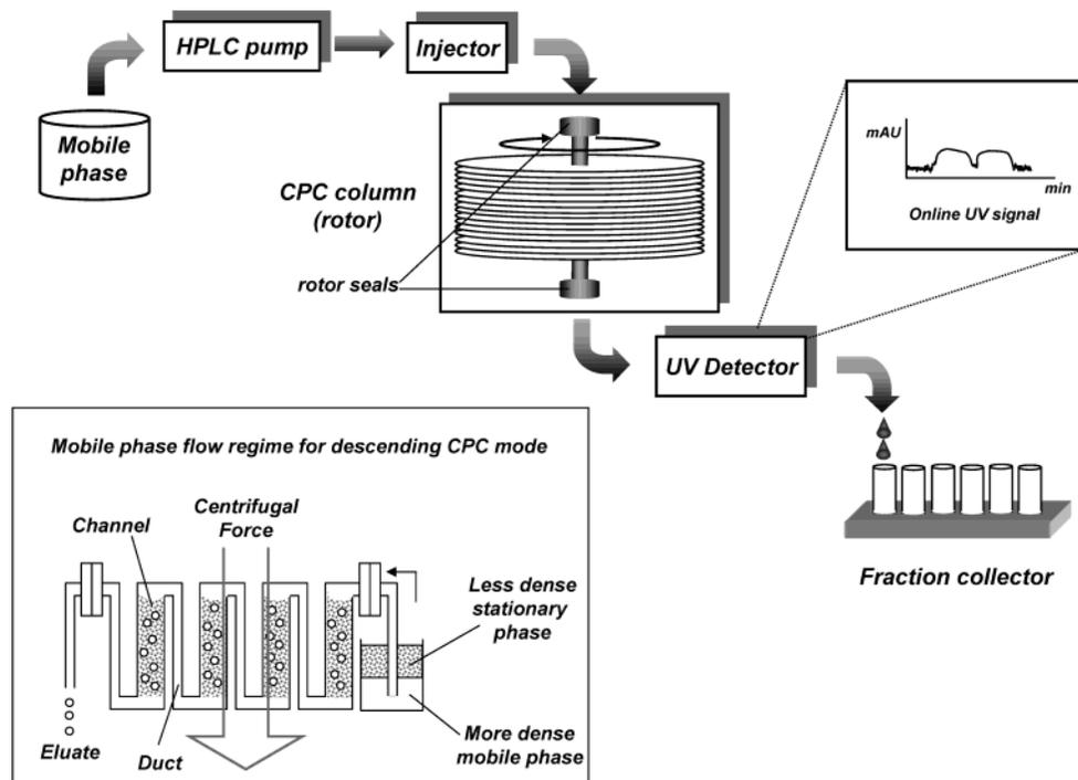
Figure 4. Schematic representation of the chromatographic equipment and (inset) the descending mode mobile-phase flow regime used for the CPC separation of the dichlorprop enantiomers.
