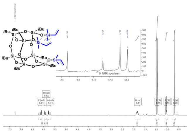
**Figure 2.** Example of the <sup>1</sup>H NMR and <sup>29</sup>Si NMR spectrum of **5** (after isolation) in CDCl<sub>3</sub> at 25 °C.
