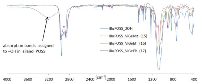
**Figure 3.** Example of the IR spectra of a reaction mixtures of 15 and 16 (after 6 h) and 17 (after 8 h) compared to disilanolisobutyl POSS.
