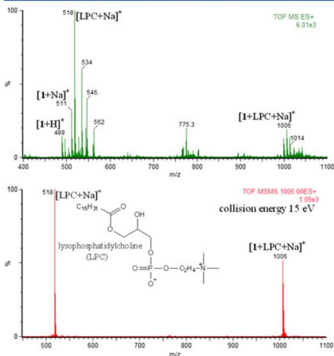
**Figure 5.** ESI mass spectra obtained for a solution containing **1** and lysophosphatidylcholine (LPC) (top: full scan mass spectrum, bottom: CID MS/MS spectrum).
