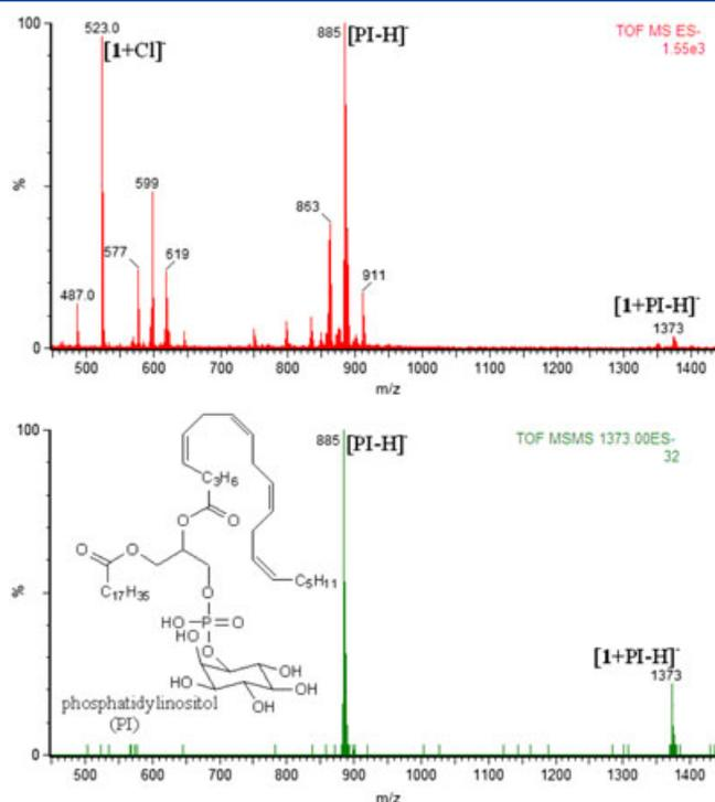
**Figure 4.** ESI mass spectra obtained for a solution containing **1** and phosphatidylinositol (PI) (top: full scan mass spectrum, bottom: CID MS/MS spectrum).
