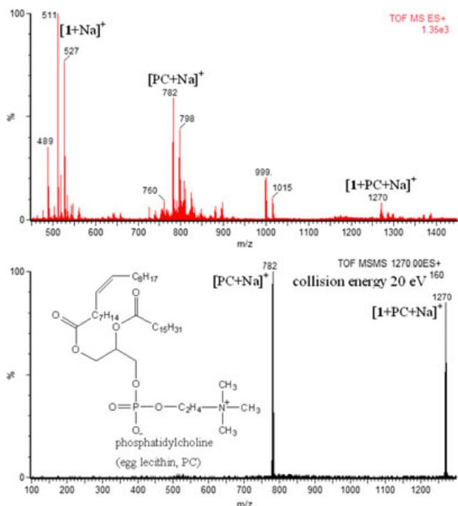
**Figure 6.** ESI mass spectra obtained for a solution containing **1** and phosphatidylcholine (PC) isolated from egg yolk (top: full scan mass spectrum, bottom: CID MS/MS spectrum).
