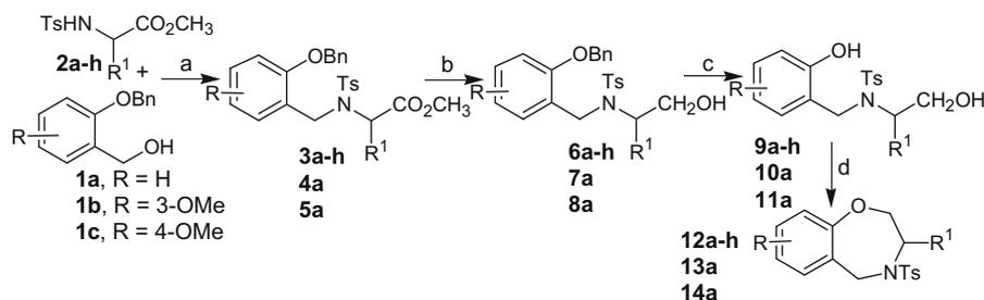
**Scheme 1.** Reagents and conditions: (a) **1a–c**, DEAD, PPh<sub>3</sub>, THF, 0 °C (2 h) to rt (10 h), N<sub>2</sub>, 60–75%; (b) LAH, THF, 0 °C, 1 h, 59–70%; (c) H<sub>2</sub>, 10% Pd/C, MeOH, rt, 2 h, 50 psi, 61–75%; (d) DEAD, PPh<sub>3</sub>, THF, 0 °C (1 h) to rt, (14 h), N<sub>2</sub>, 63–76%.
