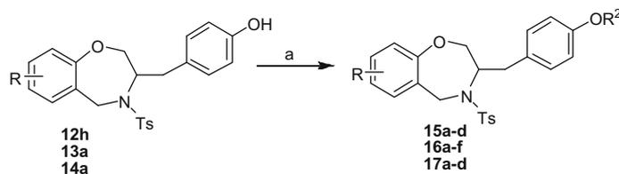
**Scheme 2.** Synthesis of amino ethyl alkyl chain derivatives with reagents and conditions: (a) anhyd  $\text{K}_2\text{CO}_3$ ,  $\text{R}^2\text{Cl}$ , dry acetone, reflux, 5 h, 60–70%.
