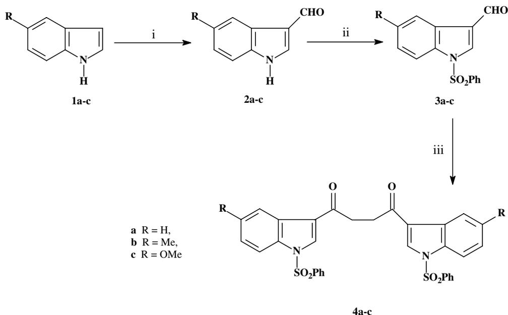
**Scheme 1.** Synthesis of intermediates **4a–c**. Reagents and condition: (i) POCl<sub>3</sub>/DMF, NaOH; (ii) NaH/THF, ClSO<sub>2</sub>Ph; (iii) thiazolium salt/EtOH, NaOAc/Divinyl sulfone, reflux.
