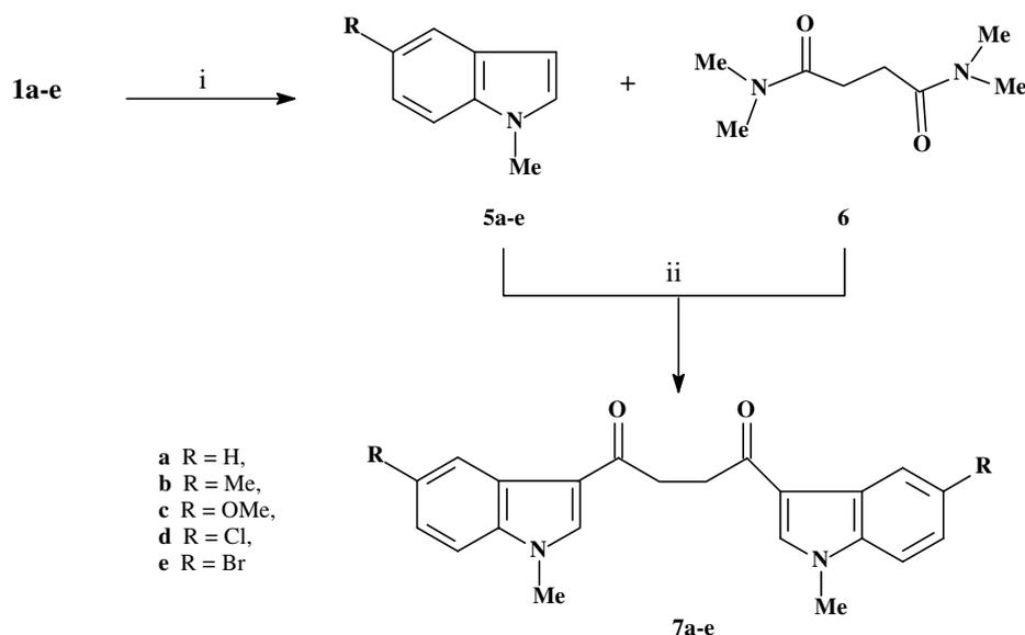
Scheme 2. Synthesis of intermediates **7a–e**. Reagents: (i) *t*-BuOK/TDA-1, benzene,  $\text{CH}_3\text{I}$ ; (ii)  $\text{POCl}_3/\text{DMF}$ .
