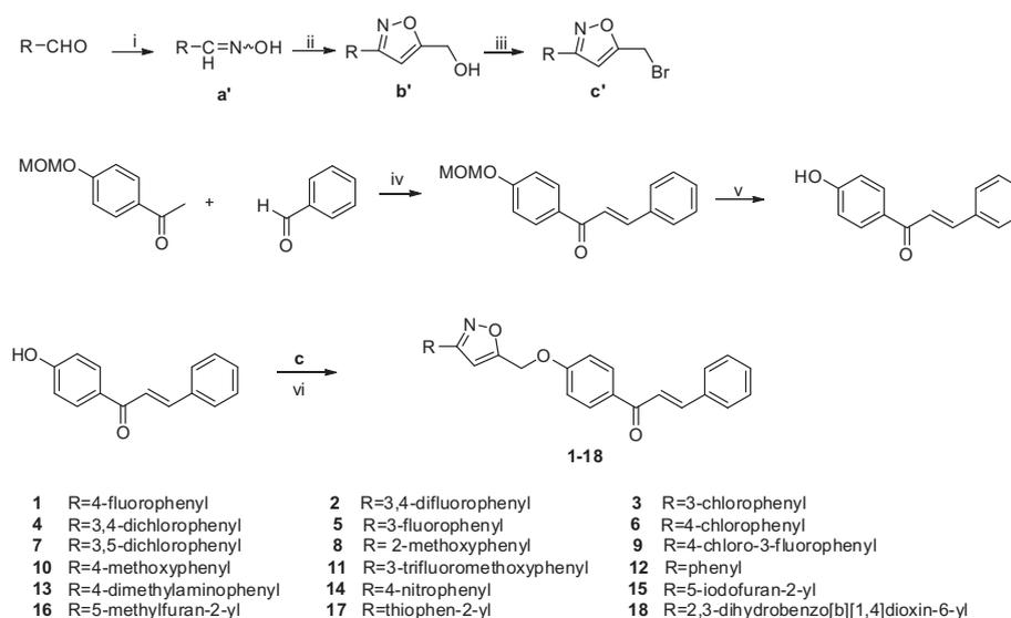
**Scheme 1.** Synthetic route for the chalcones with isoxazole. (i) NH<sub>2</sub>OH·HCl, Na<sub>2</sub>CO<sub>3</sub>, 30% methanol aqueous solution, rt (ii) NCS, propynol, triethylamine, DCM, reflux (iii) PBr<sub>3</sub>, DCM, 0 °C (iv) 10% NaOH, ethanol, rt (v) 3 M HCl, ethanol, rt (vi) K<sub>2</sub>CO<sub>3</sub>, acetone, reflux.
