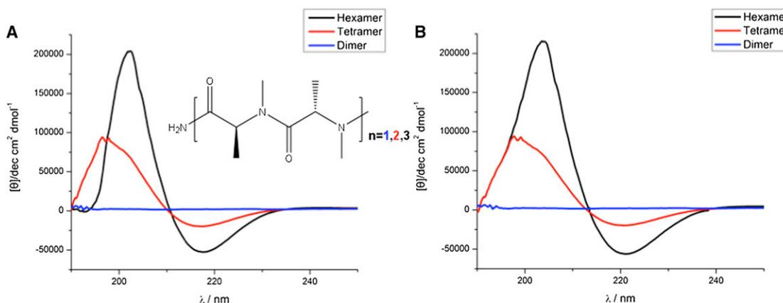
**Figure 3. CD Spectrum of the N-Methyl-Alanine Dimer, Tetramer, and Hexamer Synthesized via the Submonomer Route**
